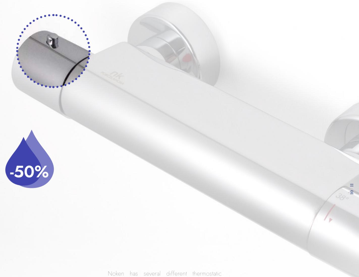
Noken has several different thermostatic faucets with ECO buttons. This mechanism enables savings of up to 50% of consumption. When the user reaches half of the flow handle's distance, it stops until the user presses the ECO button to access the thermostatic faucet's total available flow.
